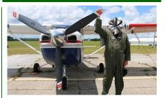
What the above member is doing looks cool for a photograph, but in reality it is very dangerous. Small aircraft engines, due to their unique design, have been know to start by moving the propeller. Even slightly. Do not touch a propeller unless you absolutely have to for preflight or repair. Also, do not allow any part of your body to pass through the propeller arc while examining the aircraft. Please remember:
